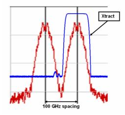
Fig 1. typical 40 Gbps duobinary channels optical spectrum and Xtract filter shape
