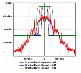
Fig 2b. typical 40 Gbps CS-RZ channel optical spectrum and Xtract filter shape
