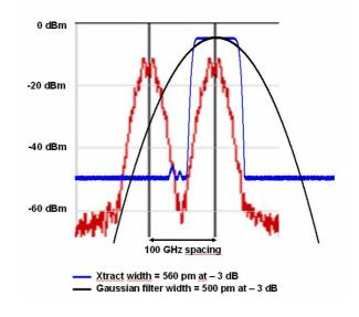
Fig 3. typical 40 Gbps duobinary channel optical spectrum with Xtract and Gaussian filter shapes
