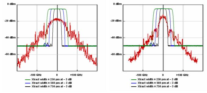
Fig 2c. typical 40 Gbps RZ-DPSK channel optical spectrum and Xtract filter shape
