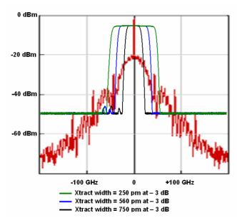
Fig 2a. typical 40 Gbps NRZ channel optical spectrum and Xtract filter shape
